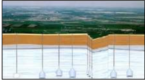
Figure 12. Salt caverns gas storage plant in Tuz Gölü.
