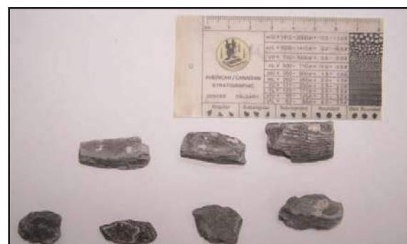
**Figure 10.** Tabular cavings reach the shakers while drilling varved shales of Osmancýk Formation.
