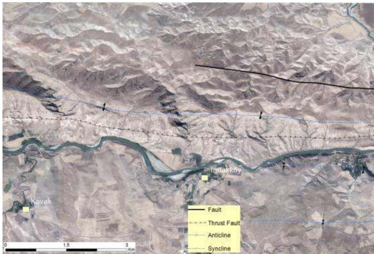
**Figure 3.** The structural lineaments of the study area overlain on an aerial photo with 0.45 cm ground resolution .
