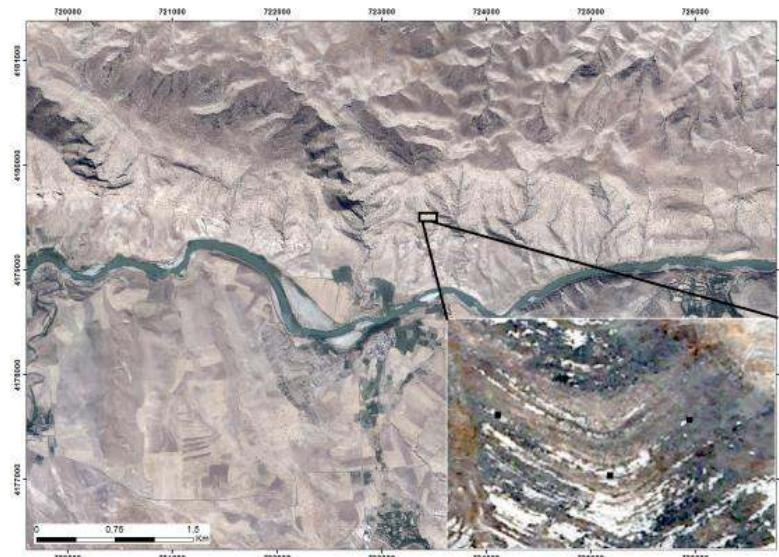
**Figure 6.** Selection of Three Vertices for strike validation using orthophotographs.
